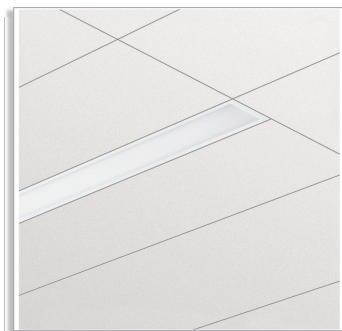
SmartForm LED BBS418 recessed luminaire, width 85 mm, with OLC micro-lens optic in polycarbonate cover (MLO-PC)
